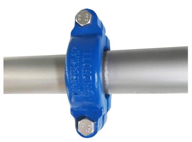
The HMP $^{\text{TM}}$ \_TE pipe coupling can be installed in a system where pipes hang on chains, parrot swings or are U-Bolted down onto pipe supports. Pipes should be anchored before and after every change of direction. The full range of HMP $^{\text{TM}}$  valves, expansion joints and energy dissipator can be manufactured with HMP $^{\text{TM}}$ \_TE coupling end connections.
